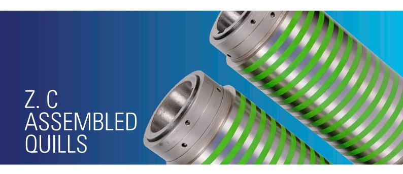
Z.C. Quills are pre-assembled cutting sets made up of circular knives, metallic spacers and vulcanized spacers. Their main application is for cutting great tonnages of slit strips which are thin and have fixed widths.. Even more the higher the quality requirements are. These complete units remain assembled from the moment tjey are mounted, during their successive sharpening and until the end of their useful cutting life.
